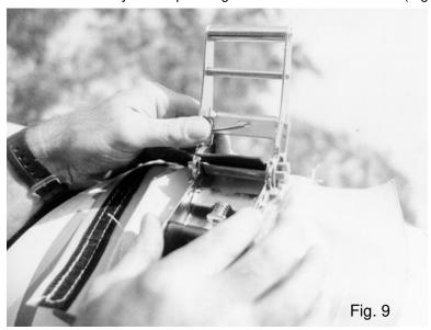
b. Pull the strap through the winder bar until the strap is taut (Fig 10).
