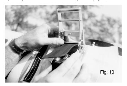
c. Tighten the strap with the ratchet until the strap is sufficiently snug to prevent the unit from moving when in use (Fig. 11). NOTE: For installation on a square boom, ensure ratchet lies against the flat surface.
