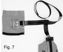
**PN 3813D1:** To mount the block and tackle to the boom weave the main attachment strap around the boom and then connect the snaphook to the dee ring. <u>Always</u> visually check that the connecting device freely engages the dee ring and the keeper/gate is completely closed. See Fig 8.
